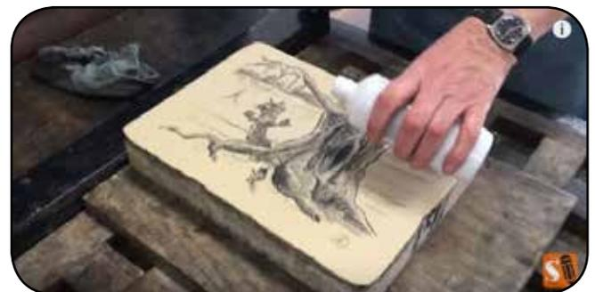
Nitric acid etches the stone where the grease is not present.
