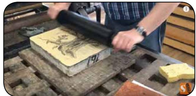
Ink is applied, paper is laid on top of the stone and put through a press.
