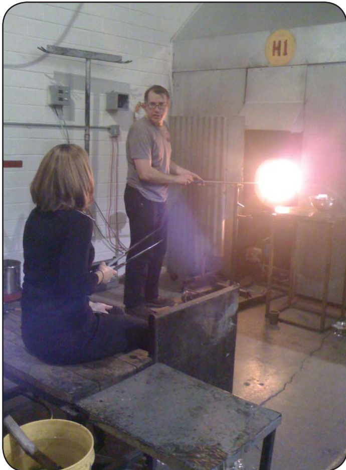
Left: Artist Daniel Schreiber prepares the glass for shaping. Above: Wendy Esposito demonstrates blowing into the glory hole; Wendy uses the jacks to shape the piece while Daniel inflates the hot glass.
