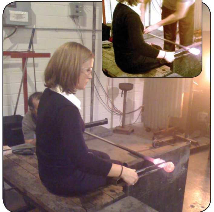
Left: Artist Daniel Schreiber prepares the glass for shaping. Above: Wendy Esposito demonstrates blowing into the glory hole; Wendy uses the jacks to shape the piece while Daniel inflates the hot glass.
